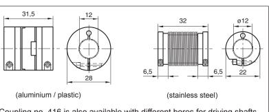
Coupling no. 416 is also available with different bores for driving shafts with diameters other than 12 mm.
