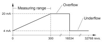
Note: If the measuring range cannot be found directly due to sensor shaft rotation (as the sensor system is in the overflow or underflow range), the rotary encoder can be set to the zero point with the MFPs.
